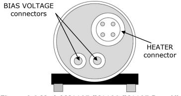
Figure 3.2 Model M1125/M1130/M1135 Rear View
