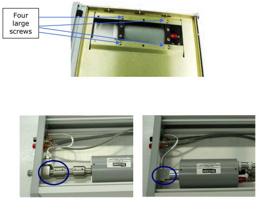
Figure 5.2 Location of Power Splitter in the F1125/F1130 and F1135
