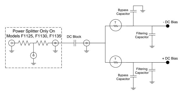
Figure 4.1 Simplified Schematic of RF Power Standards
