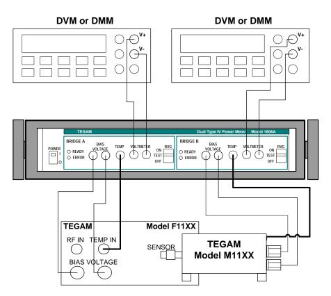
Figure 5.6 Connection Diagram for Characterizing a Working Standard
