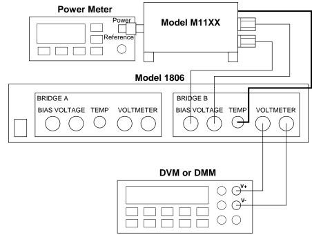
Figure 1.5 Measuring a 50 MHz Reference Output on a Power Meter using a Terminating RF Power Standard (Model M1125, M1130, M1135)
